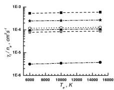
**Fig. 1.** The ratio of the total width to the electron density  $(n_e = 10^{14} \text{cm}^3)$  as a function of the electron temperature  $T_e$  for the studied Ar I lines ( $\blacksquare$  522.1, \* 549.6,  $\circ$ 518.6,  $\blacktriangle$ 603.2, \*560.7,  $\circ$ 696.6 nm)
