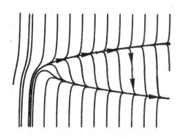
Example of changing asymptotic behaviour: Solutions of the differential equation  $dY/dX = Y^2-X$ .
