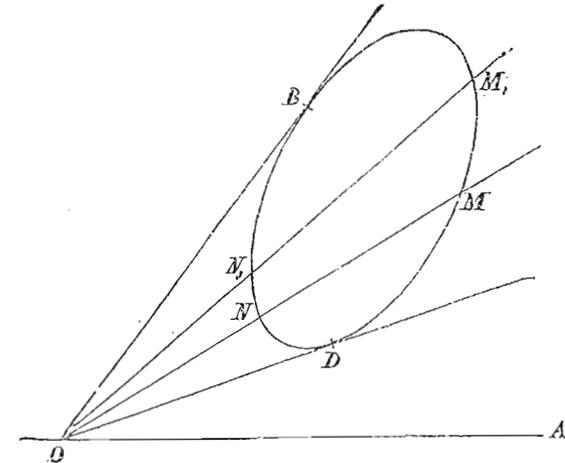
$$\text{Fl. } BNDMB = \lim \frac{\Sigma(RR_1 - rr_1) \sin(t_1 - t)}{2} = \int_y^{\delta} \frac{R^2 - r^2}{2} dt, \quad (47)$$
