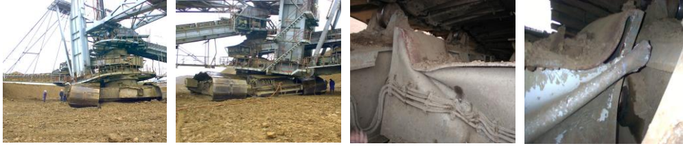
Figure 1. Position of conveyer and the outlook of the damaged spot
