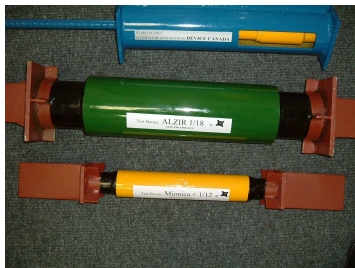
Figure 3. Typical dampers of DC 90 system
