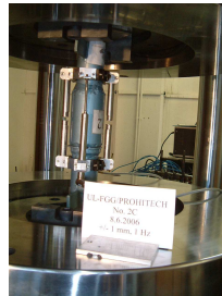
Figure 4. Damper testing on MTS machine
