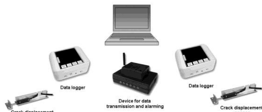
Figure 1. System for continuous remote crack monitoring
