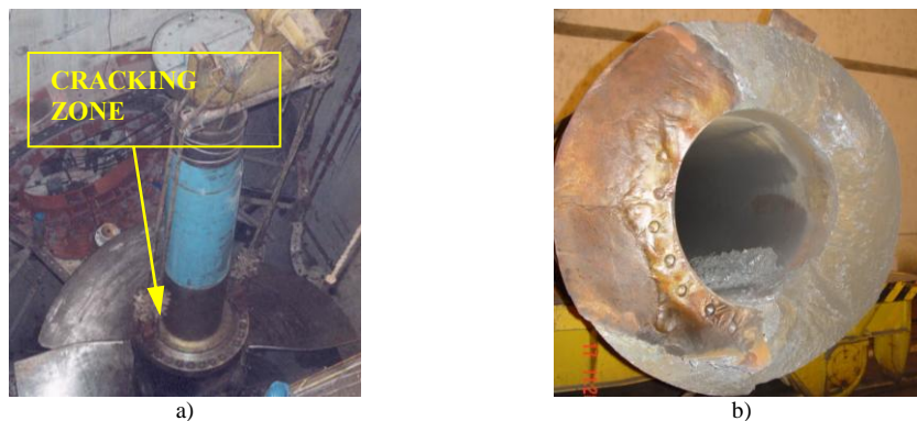
Figure 2. a) turbine shaft with runner during assembling in the bulb, b) fractured surface
