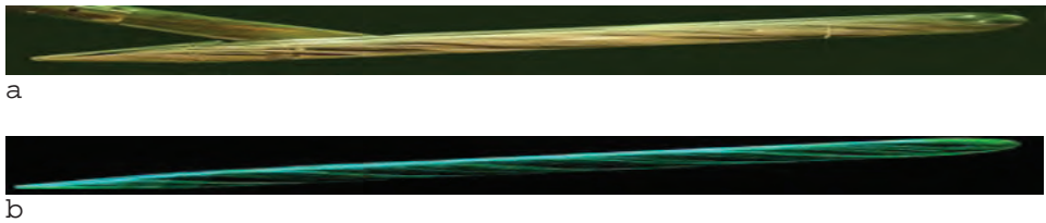
Figure 12: Flow pattern on the model obtained by the experiment (a) and by the simulation of the flow for M_\infty = 0.3 and \alpha = 8^\circ (side view) (b) [21].
