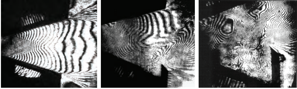
Fig. 28. Holographic interferograms for 2D supersonic nozzle without and with three barriers
