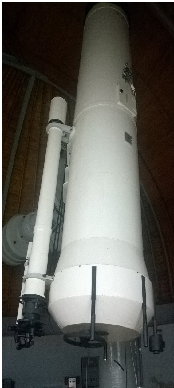
Figure 1: The Schmidt-camera 50/70 cm (NAO Rozhen, Bulgaria).
