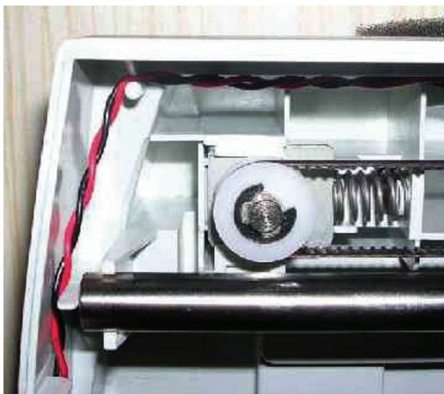
Figure 6. The tightening pulley, the cogged rubber belt, mounted of the guide.
